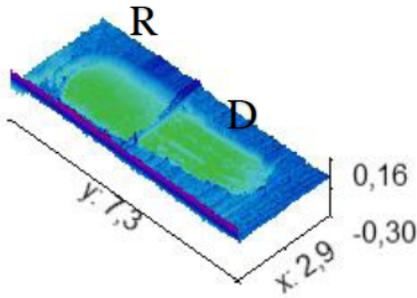
**Figure 4:** Example of wear pattern obtained from 3D images obtained with the laser profilometer, showing the oval shape of the track, the interface, the major depth at the interface. D: the dentin, RM: the resin material. Note the distinct transition in depth of wear from the enamel to the bonded interface and resin composite.
