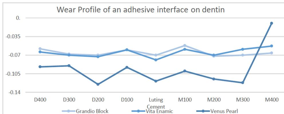
**Graph 4:** Comparison between the wear profiles obtained at the luting cement interface (midpoint) and at 100 $\mu$ m, 200  $\mu$ m, 300  $\mu$ m, 400  $\mu$ m at both dentin and restorative material sides. D: the dentin, M: the restorative material. The greatest wear rate is located at the dentin side and a difference between CAD-CAM materials and nano hybrid composite is also observed.
