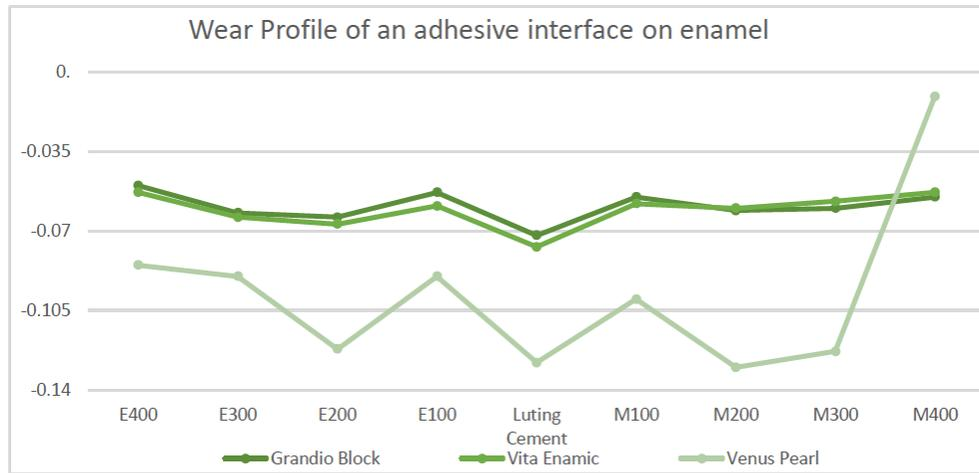
**Graph 3:** Comparison between the wear profiles obtained at the luting cement interface (midpoint) and at 100 $\mu$ m, 200  $\mu$ m, 300  $\mu$ m, 400  $\mu$ m at both enamel and restorative material sides. E: the enamel, M: restorative material. It is evident the minimal wear of the enamel side and the great difference in wear rate between CAD-CAM materials and the nano hybrid composite. Note the profile obtained before and after the luting cement midpoint, where the lowest peaks are located.
