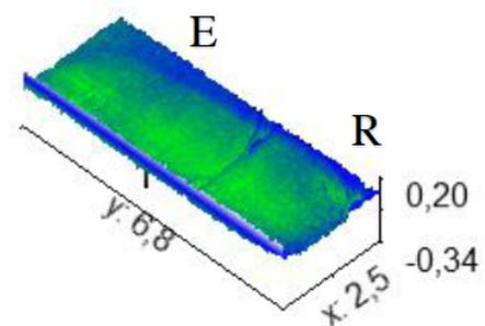
**Figure 3:** Example of wear pattern of an enamel-material specimen, showing the oval shape of the wear track, the interface and the major depth at the interface. E: the enamel, RM: the resin material. Note the distinct transition in depth of wear from the enamel to the bonded interface and resin composite.
