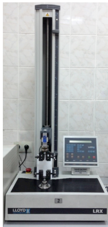
Figure 2: Three point bending test was perform using computer-controlled Universal Testing Machine at a cross-head speed of 1mm/min.
