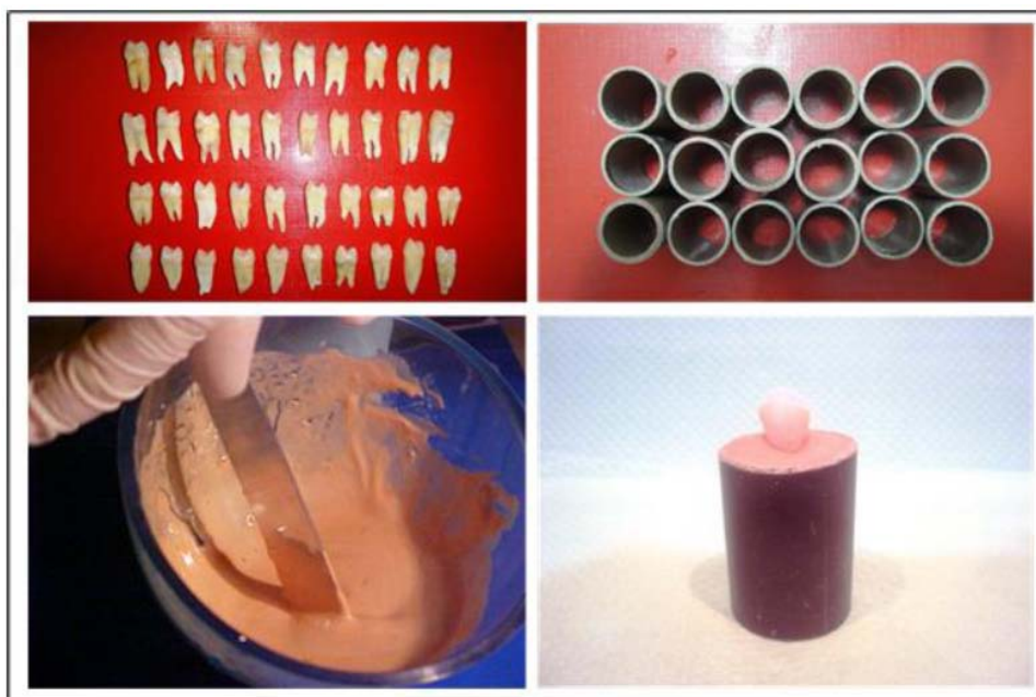
Figure 1: Premolars; tubes PVC; special plaster; specimen.
