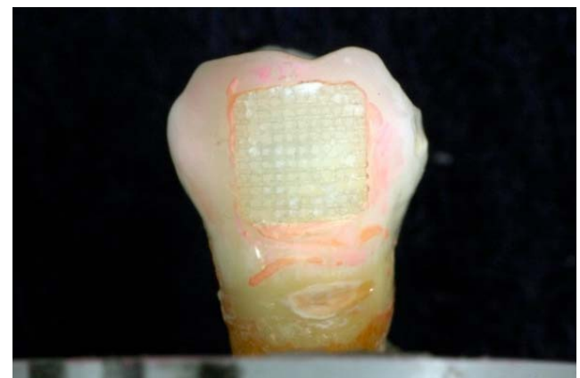
Figure 3: Adhesive failure pattern: material/bracket adhesive.
