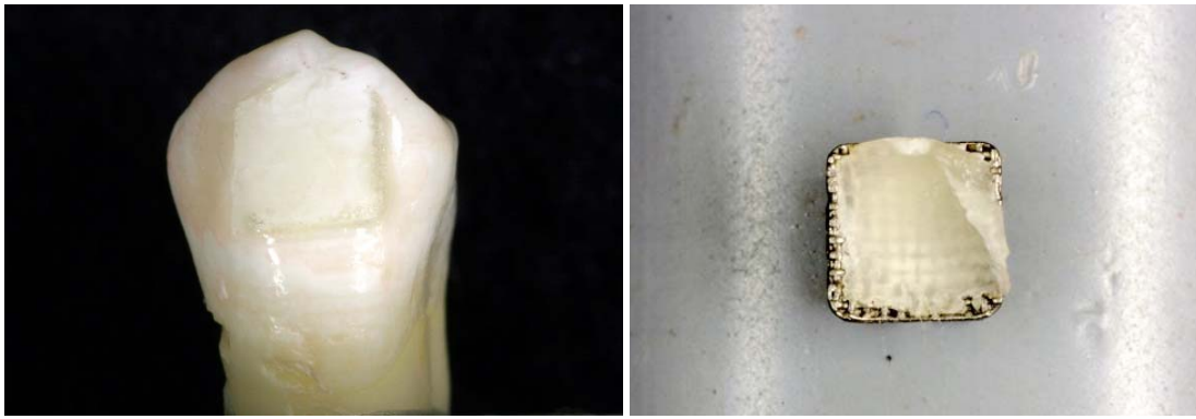
Figure 4: Adhesive failure pattern: material/tooth adhesive (the enamel surface presented no adhesive remnant; the adhesive remained adhered to the bracket).
