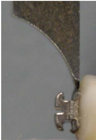
Figure 1: Chisel extremity positioned at the bracket/enamel interface during the SBS test.
