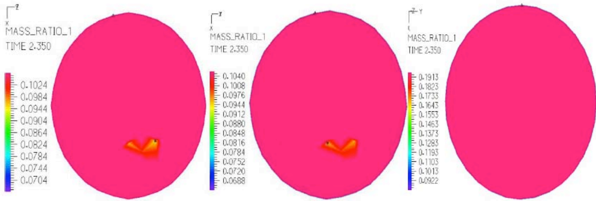
Figure 16: Mass ratio band plot at ICA entrance and end systole ( t/t_p=2.35 ). From left to right: Mooney-Rivlin, linear elastic and solid models.
