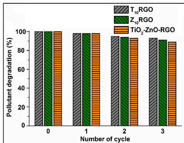
Figure 7: Organic pollutant decontamination efficiency at different cycles.
