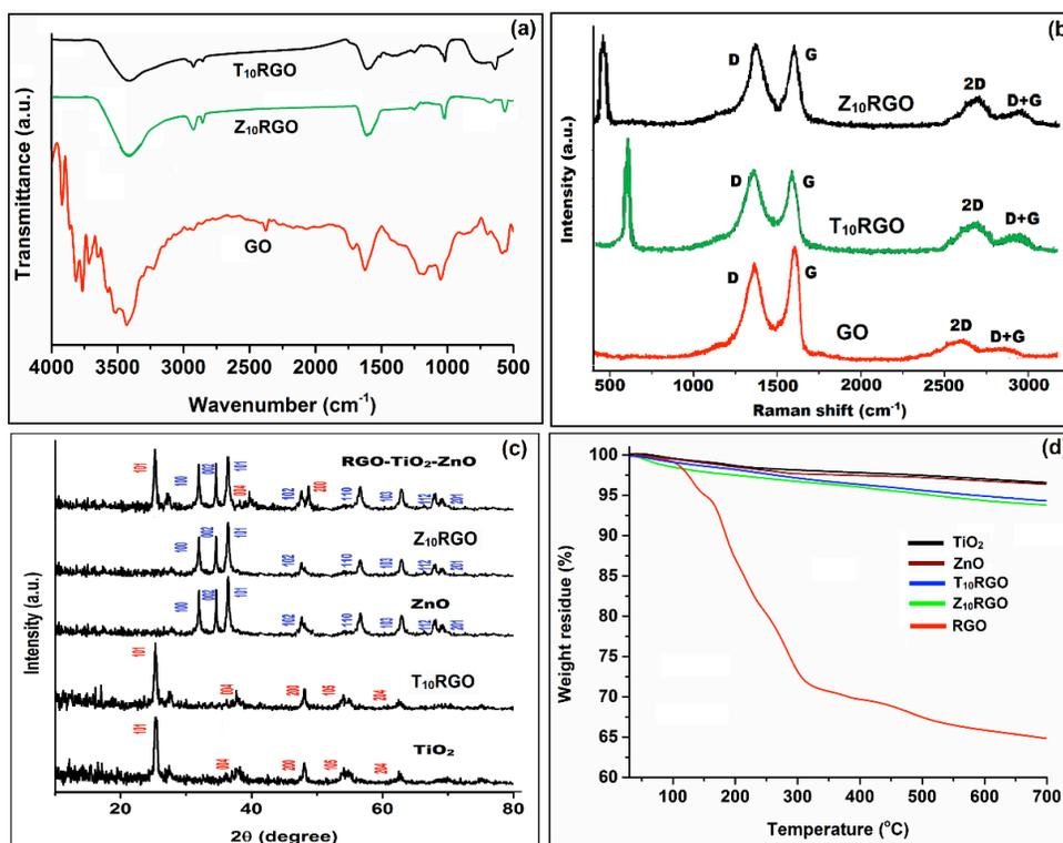
**Figure 1:** (a) FTIR and (b) Raman spectra of GO, T<sub>10</sub>RGO and Z<sub>10</sub>RGO nanohybrid; (c) XRD patterns of TiO<sub>2</sub> nanoparticles, ZnO nanoparticles, T<sub>10</sub>RGO, Z<sub>10</sub>RGO and TiO<sub>2</sub>-ZnO-RGO nanohybrid, and (d) TGA thermograms of TiO<sub>2</sub> nanoparticles, ZnO nanoparticles, RGO, T<sub>10</sub>RGO and Z<sub>10</sub>RGO.
