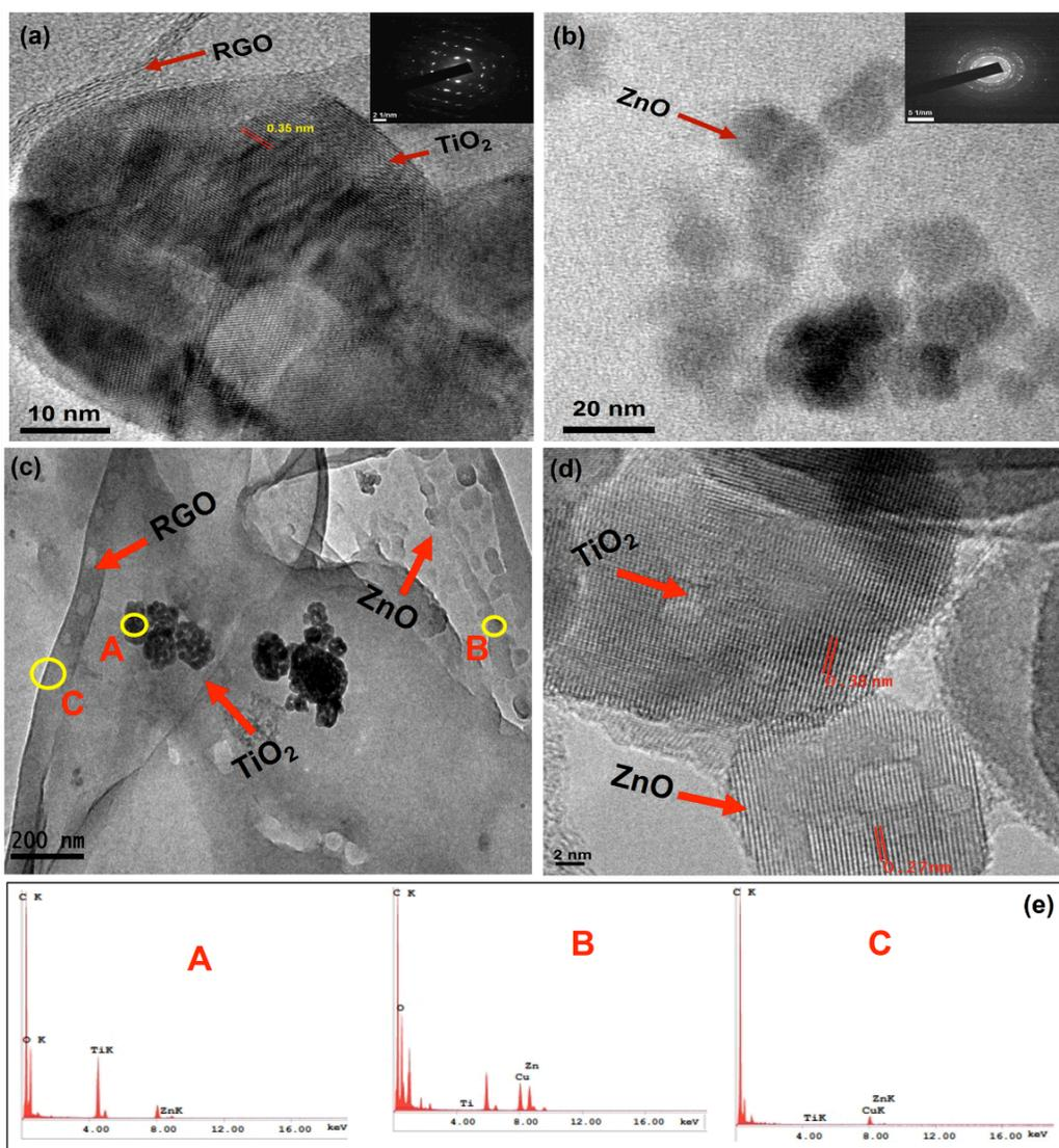
**Figure 2:** HRTEM images of (a) T<sub>5</sub>RGO, (b) Z<sub>5</sub>RGO, (c) and (d) TiO<sub>2</sub>-ZnO-RGO nanohybrid; and (e) EDS of TiO<sub>2</sub>-ZnO-RGO nanohybrid.
