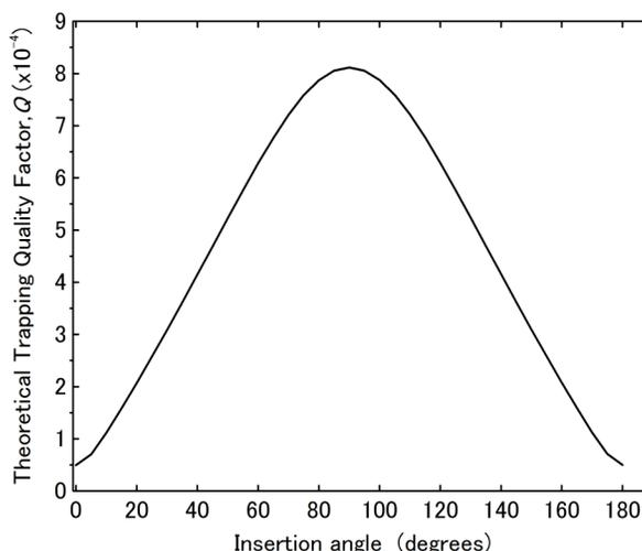
**Figure 5:** Theoretical trapping quality,  $Q$ , for various angle insertions.
