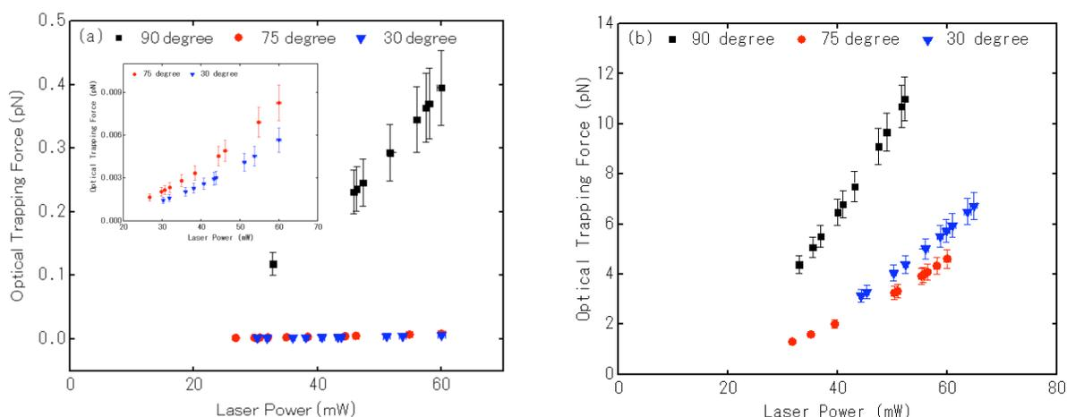
**Figure 4:** Optical trapping force as a function of the trapping laser power for, (a) 900-nm polystyrene beads and (b) 3-µm PMMA beads, for various insertion angle degrees into the sample chamber. Inset: the trapping force for insertion angle 75 and 30 degrees, for the 900-nm polystyrene beads. The x-error and the y-error correspond to the standard deviation of the trapping force measurement.
