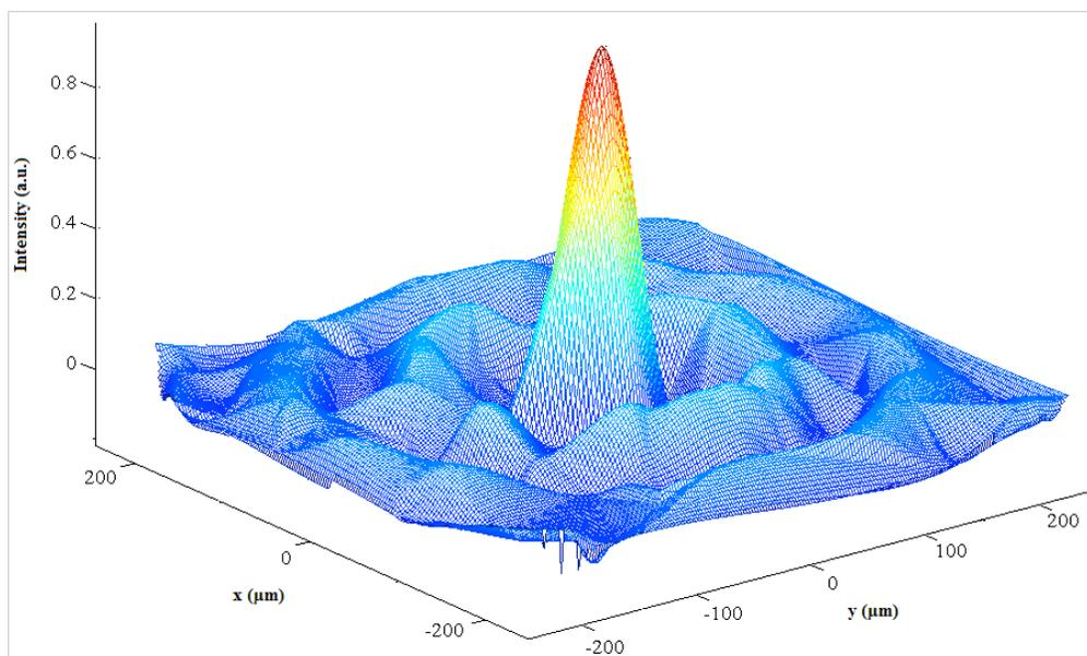
**Figure 2:** The theoretical output beam profile at the outlet of the optical fiber, which is used to create the optical fiber tweezers.
