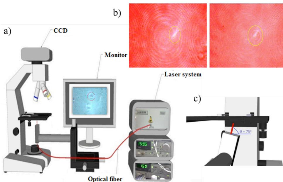
**Figure 1:** Experimental set up. (a) A schematic diagram of the fiber trapping system. (b) Some representative results: The beam entry was close to the cover glass and formed an aura, as can be seen in the left image. The right image shows the trapped particle by the optical forces exerted on a 3- $\mu\text{m}$  PMMA bead. (c) A schematic diagram of the insertion angle measurements.
