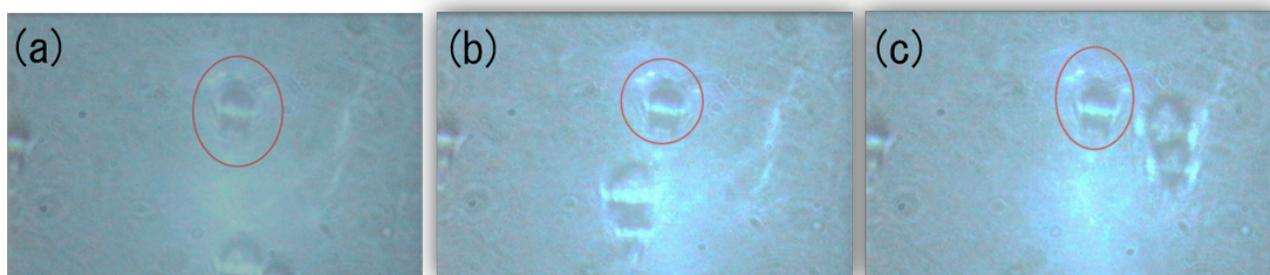
**Figure 3:** A series of single frames of trapped 3- $\mu\text{m}$  PMMA bead using the fiber optical tweezers. The red cycle represents the position of the trapped bead. The optical fiber was inclined at 90 degrees to the sample chamber.
