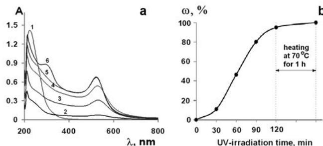
**Figure 1:** The kinetics of gold nanoparticles formation in 3 wt.% chitosan solutions containing 2 wt.% acetic acid with initial concentration of  $\text{HAuCl}_4$  3 wt.% by UV-irradiation: (a) the changes in absorption spectra of solutions; (b) the change of the Au NPs relative content ( $\omega$ , %) in the chitosan solution during UV-irradiation and heat treatment.
