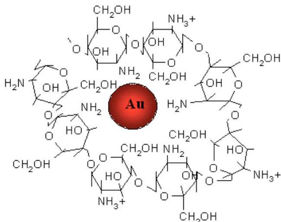
**Figure 3:** Stabilization of gold nanoparticles by chitosan macromolecules in its solution.
