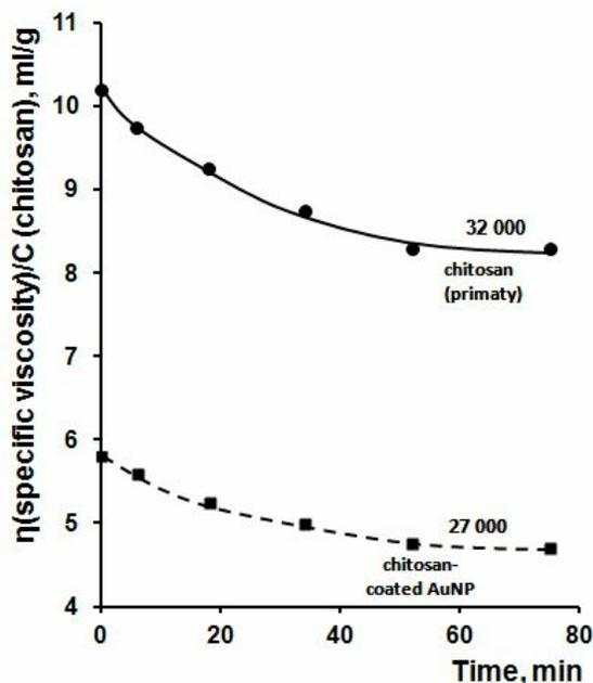
**Figure 4:** Variation with time in the reduced viscosity value of the solutions of chitosan and chitosan-coated AuNP treated with pancreatine.
