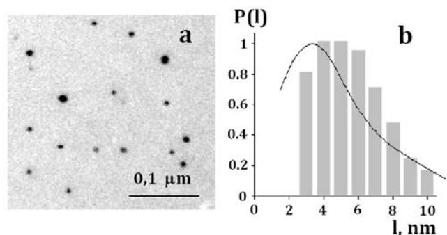
**Figure 2:** TEM images of gold nanoparticles (a). The nanoparticles size distribution according from to TEM (histogram) and SAXS (curve) (b).
