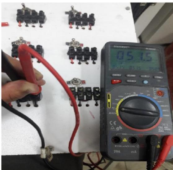
**Figure 4:** Output voltage measurement.
