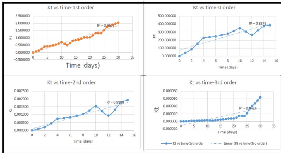
Figure 6: Data and Kinetic Models for the Second Group MFCs: MFC 4, 5, and 6.
