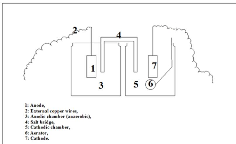
**Figure 1:** Schematic of DS-MFC used.
