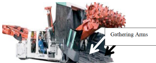
Figure 1: Typical 600 kW underground CM (courtesy of Sandvik Mining – Netherlands).
