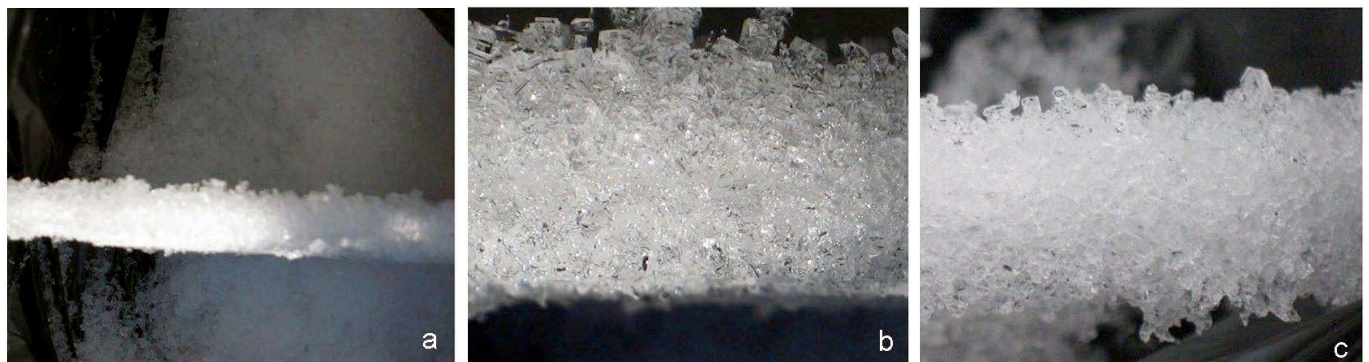
Figure 5: Subliminal adfreezing of depth hoarfrost crystals into a plate (a), formation of asperities on the plate in the process of depth hoarfrost crystal growth (b, c).
