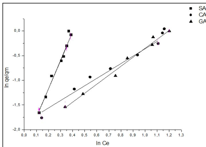
**Figure 9:** Adsorption isotherms from the Toth model. Conditions:  $T = 24 \pm 2^\circ\text{C}$ , adsorbent amount = 0.050 g,  $\text{pH} = 3$ .
