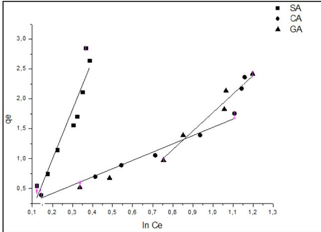
Figure 7: Adsorption isotherms from the Temkin model. Conditions: T = 24±2°C, adsorbent amount = 0.050 g, pH = 3.
