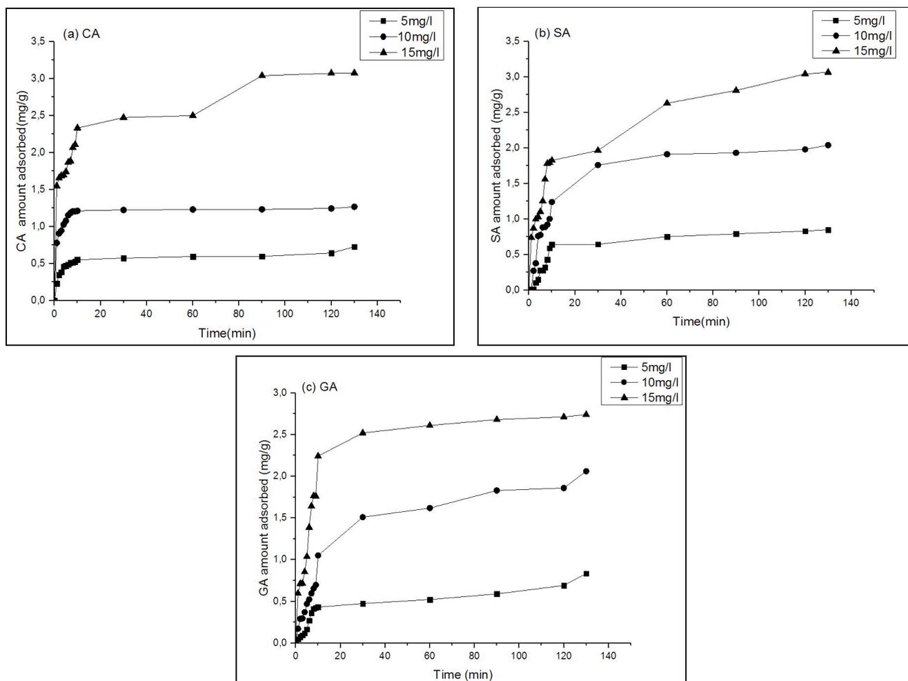
**Figure 4:** Effect of the initial concentration of (a) CA, (b) SA and (c) GA on the adsorption efficiency. Conditions:  $T = 24 \pm 2^\circ\text{C}$ , adsorbent amount = 0.050 g,  $\text{pH} = 3$ .
