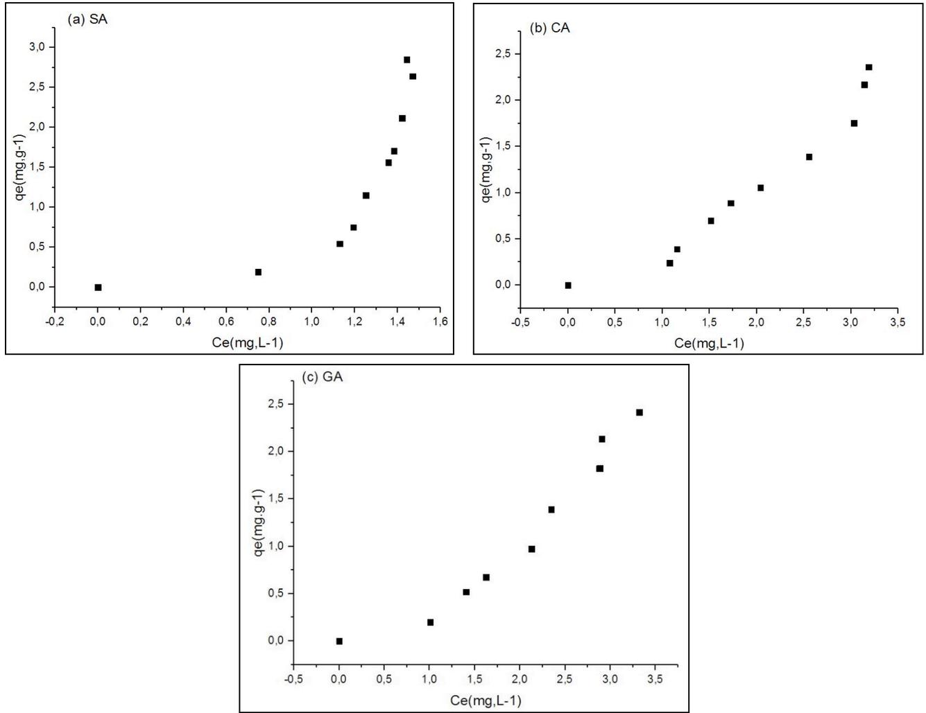
Figure 5: Equilibrium adsorption isotherms, measured at temperature 24±2°C. (a) SA, (b) CA and (c) GA.
