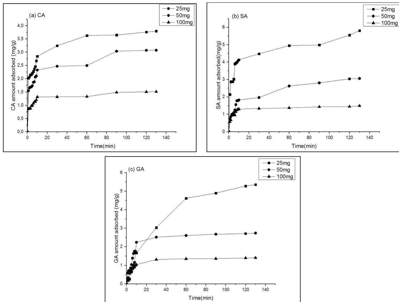
**Figure 3:** Effect of the activated carbon mass on the adsorption capacity of (a) Clofibric acid, (b) Salicylic acid and (c) Gallic acid. Conditions: adsorbate concentration =  $15 \text{ mg/dm}^3$ ,  $T = 24 \pm 2^\circ\text{C}$ ,  $\text{pH} = 3$ .
