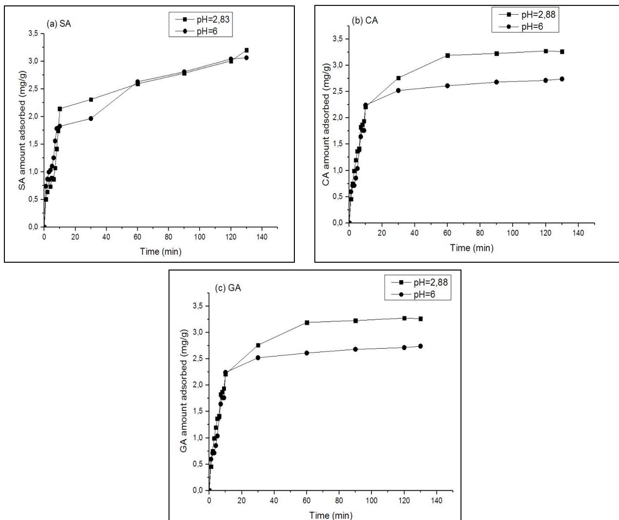
**Figure 2:** Kinetics results (a) SA, (b) CA and (c) GA for pH = 3 and 6. Conditions: adsorbent dosage = 0.05g, adsorbent concentration = 15 mg/dm<sup>3</sup>, T = 24±2°C.
