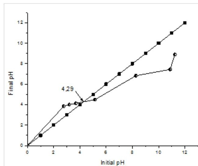
**Figure 1:** Determination of the point zero of charge of the activated carbon.
