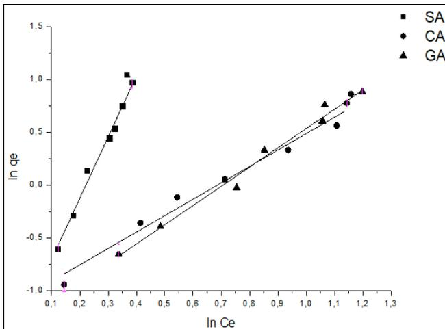
Figure 6: Adsorption isotherms from the Freundlich model. Conditions: T = 24±2°C, adsorbent amount = 0.050 g, pH = 3.
