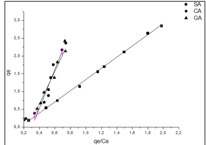
Figure 8: Adsorption isotherms from the Langmuir model. Conditions: T = 24±2°C, adsorbent amount = 0.050 g, pH = 3.
