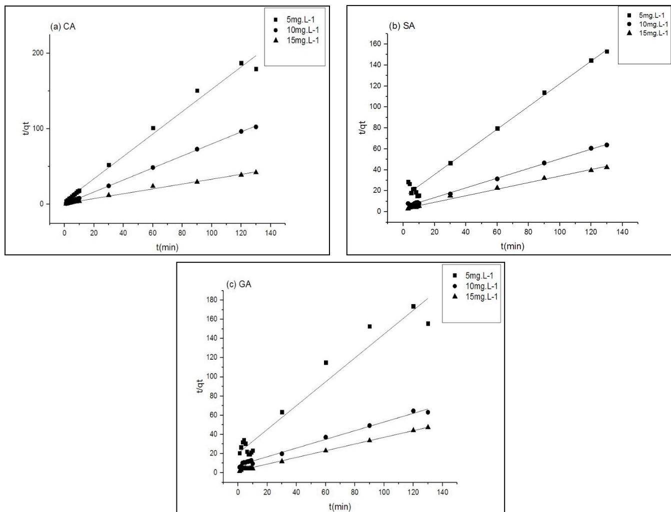
Figure 10: Pseudo-second order kinetics fits. Conditions:  $T = 24 \pm 2^\circ\text{C}$ , adsorbent amount = 0.050 g, pH = 3.
