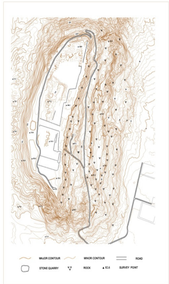
Figure 1: Stereo topographical Survey.
