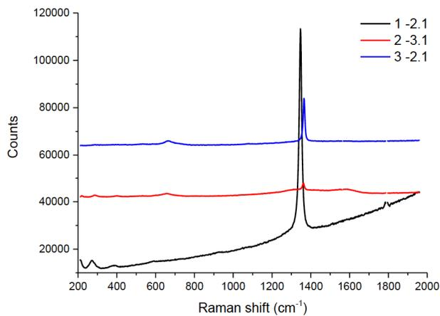
**Figure 4:** Raman spectra of: (1) composite h-BN–Fe<sub>3</sub>O<sub>4</sub> synthesized in presence of h-BN by co-precipitation of iron(II) and iron(III) compounds; (2) h-BN–Fe composite obtained by iron deposition on boron nitride using iron(O) pentacarbonyl; and (3) h-BN–Fe<sub>3</sub>O<sub>4</sub> composite obtained by using iron(O) pentacarbonyl.
