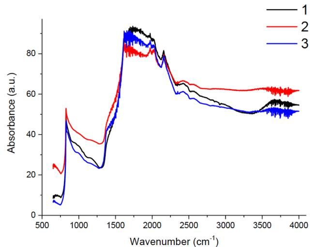
**Figure 5:** FTIR spectra of: (1) composite h-BN–Fe<sub>3</sub>O<sub>4</sub> obtained in presence of h-BN by co-precipitation of iron(II) and iron(III) compounds; (2) h-BN–Fe composite obtained by iron deposition on boron nitride using iron(O) pentacarbonyl; and (3) h-BN–Fe<sub>3</sub>O<sub>4</sub> composite obtained by using iron(O) pentacarbonyl.
