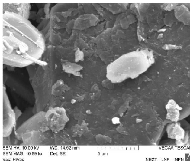
**Figure 2:** SEM image of h-BN-Fe composite obtained by iron deposition on boron nitride using iron(O) pentacarbonyl.
