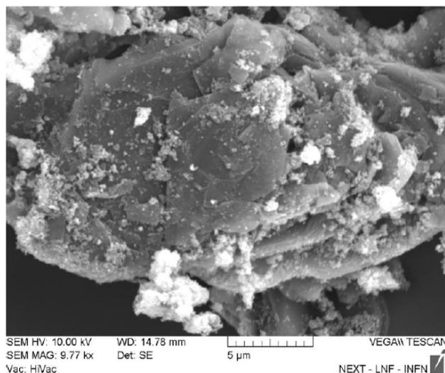
**Figure 1:** SEM image of h-BN- $\text{Fe}_3\text{O}_4$  composite obtained by co-precipitation of iron(II) and iron(III) compounds in presence of h-BN.
