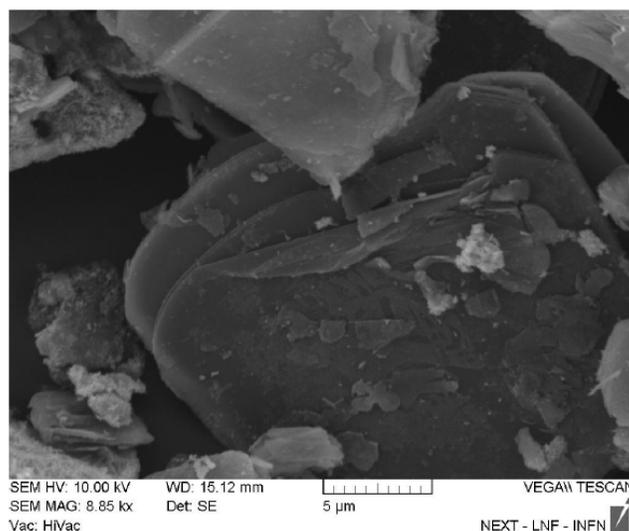
**Figure 3:** SEM image of h-BN- $\text{Fe}_3\text{O}_4$  composite obtained by using iron(O) pentacarbonyl.
