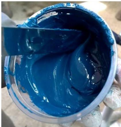
**Figure 8:** Mixture of adhesive and hardener.
