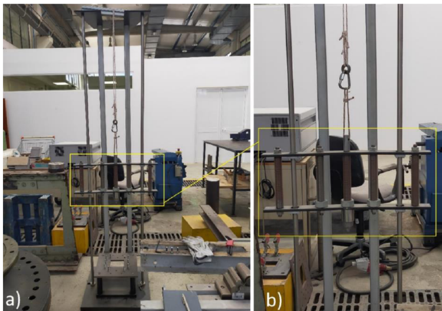
Figure 2: Drop weight impact test: (a) setup and (b) impactor tip and mass detail.
