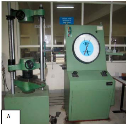
Figure 5: (A) shows Universal testing machine (B) Experimental setup.
