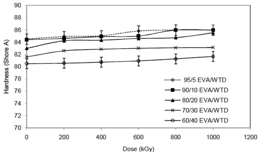
**Figure 3:** Effect of pre irradiation of WTD on the hardness of EVA/WTD blends.
