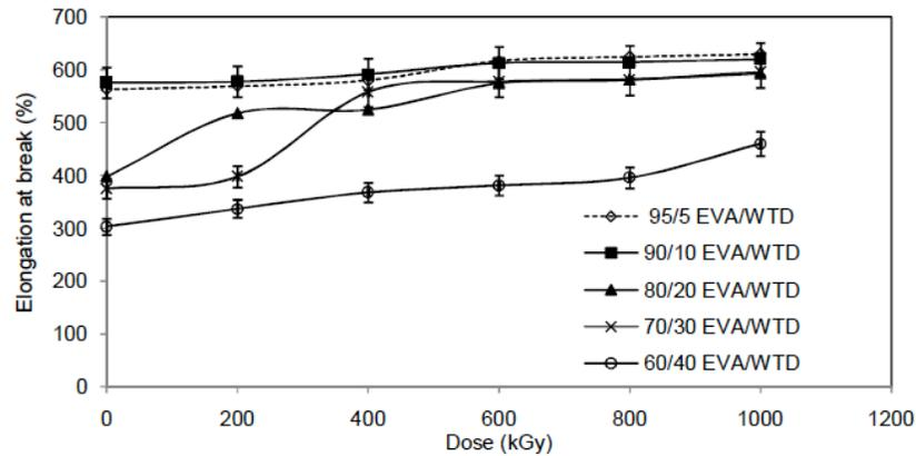
**Figure 2:** Effect of pre irradiation of WTD on the Eb of EVA/WTD blends.
