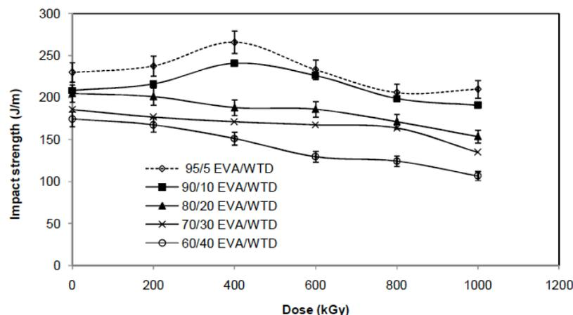
Figure 4: Effect of pre irradiation of WTD on the impact strength of EVA/WTD blends
