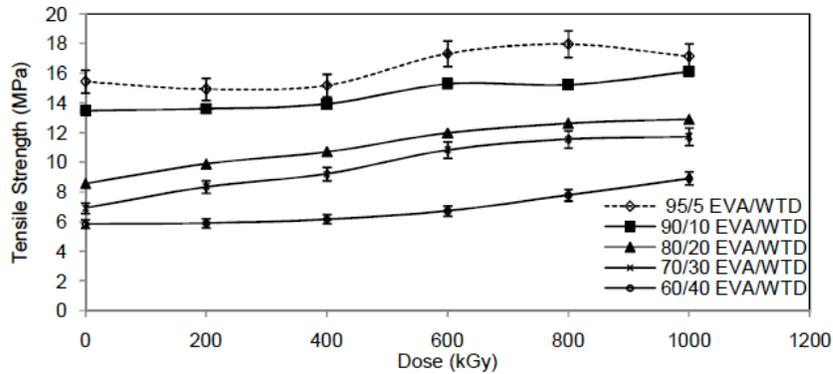
**Figure 1:** Effect of pre irradiation of WTD on the Ts of EVA/WTD blends.
