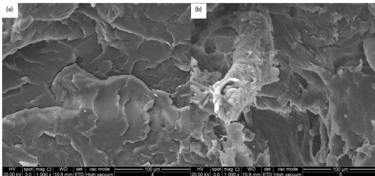
**Figure 7:** SEM photomicrographs of 80/20 EVA/WTD blend (a) 0kGy (b) 800 kGy (magnification x1000).
