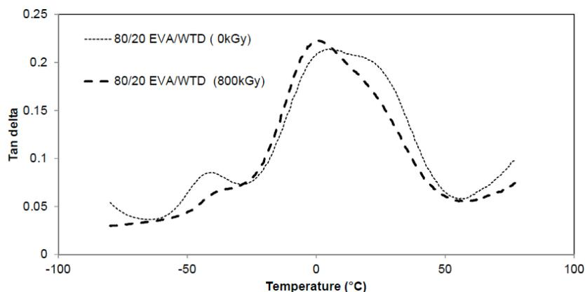
**Figure 5:** Effect of pre irradiation of WTD on the temperature dependence of the  $\tan \delta$  of 80/20 EVA/WTD blend.
