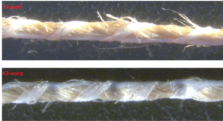
Figure 9: Surface of yarns, used in jute fabric (K3).
