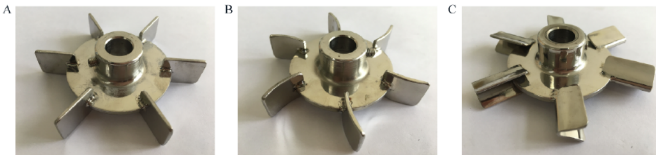
Figure 1: Three agitators with different blade shapes. (A) Six-flat-blade disc turbine. (B) Six-curved-blade disc turbine. (C) Six-arrow-blade disc turbine.
