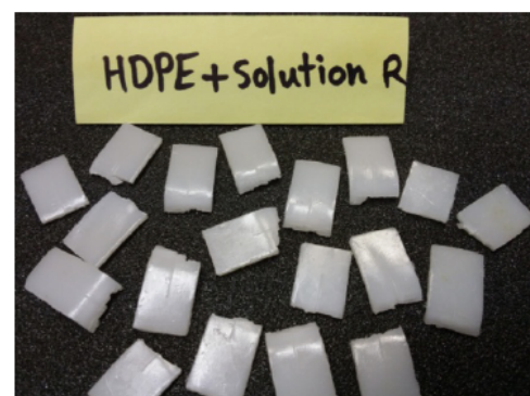
Figure 4: Cracking of all samples of commercial HDPE (HDPE-C) after the course of ESCR test.
