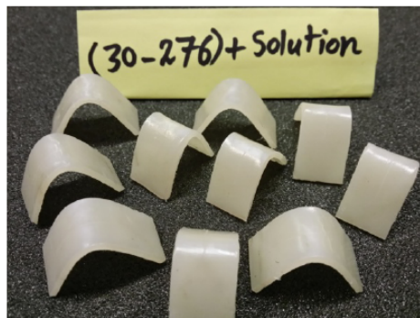
Figure 3: Appearance of homemade HDPE (HDPE-276-30 and HDPE-276-40) after the course of ESCR test.
