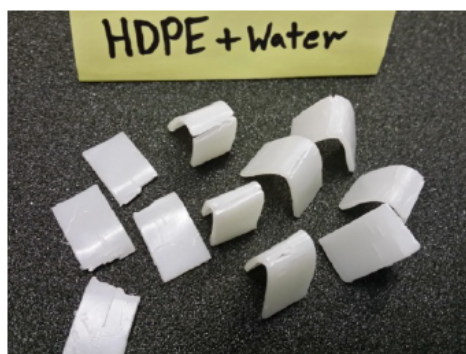
Figure 6: Cracking of the samples of commercial HDPE (HDPE-C) after the course of ESCR test with water.
