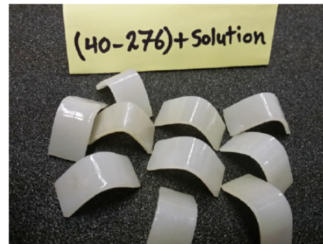
Figure 3: Appearance of homemade HDPE (HDPE-276-30 and HDPE-276-40) after the course of ESCR test.
