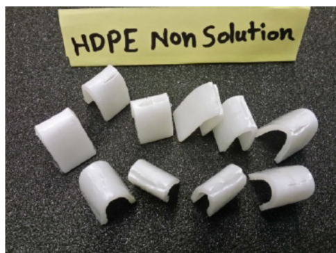
Figure 5: Cracking of some of the samples of commercial HDPE (HDPE-C) after the course of ESCR test without using any solution.
