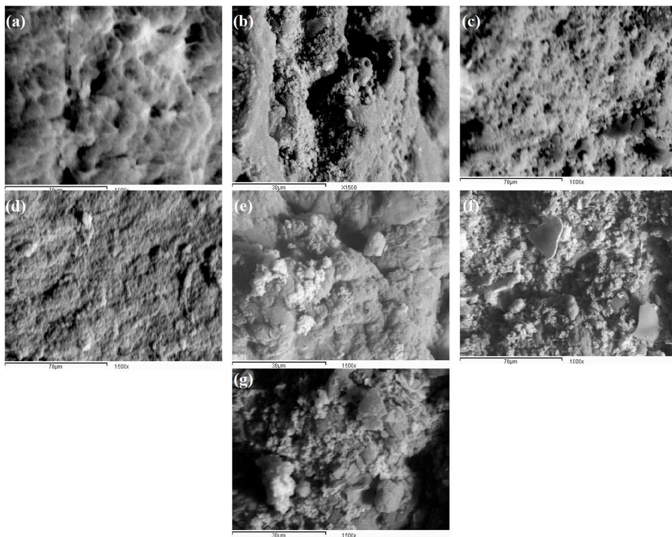
**Figure 3:** SEM microphotographs of (a) PGMA-*g*-Pectin hydrogel (0.25 mol GMA), (b) PGMA-*g*-Pectin hydrogel (0.5 mol GMA), (c) PGMA-*g*-Pectin hydrogel (0.75 mol GMA), (d) PGMA-*g*-Pectin hydrogel (1 mol GMA), (e) PGMA-*g*-Pectin-Urease (0.75 mol GMA, 1 mg urease), (f) PGMA-*g*-Pectin-Urease (0.75 mol GMA, 5 mg urease), and (g) PGMA-*g*-Pectin-Urease (0.75 mol GMA, 10 mg urease).
