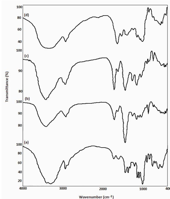
**Figure 2:** FT-IR of (a) Pectin, (b) PGMA-g-Pectin, (c) PGMA-g-Pectin-Urease, and (d) Urease.
