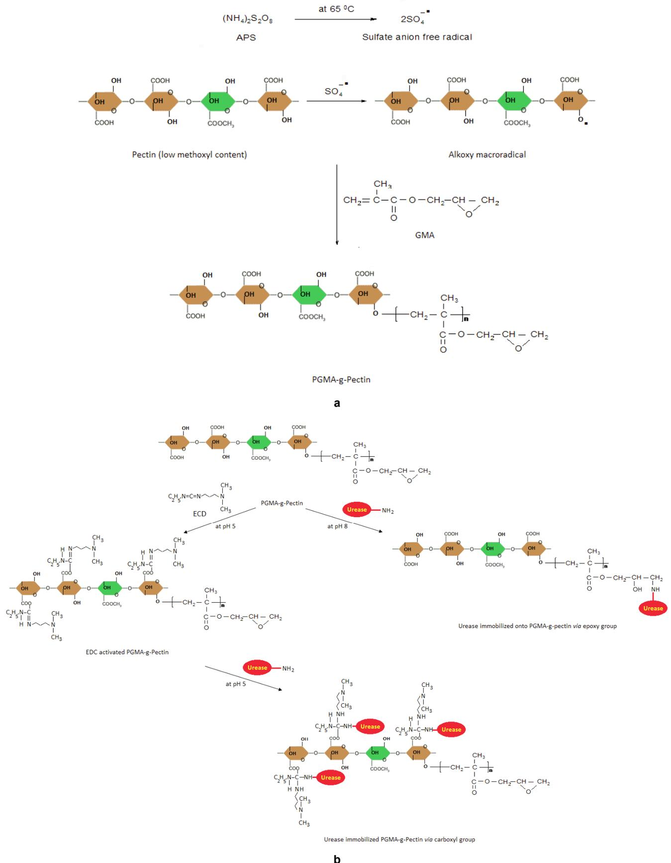
**Figure 1:** Schematic representation of (a) the grafting reaction mechanism of the PGMA on pectin and (b) the immobilization of urease onto PGM-g-pectin via carboxyl and epoxy groups.
