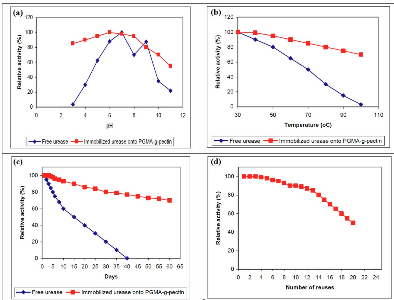
**Figure 4:** Studies of different parameters affecting urease activity: Optimum (a) pH and (b) temperature, (c) storage stability of free and immobilized urease onto PGMA-g-Pectin hydrogel at 4°C and (d) reusability of immobilized urease onto PGMA-g-Pectin hydrogel in repeated hydrolysis of urea.
