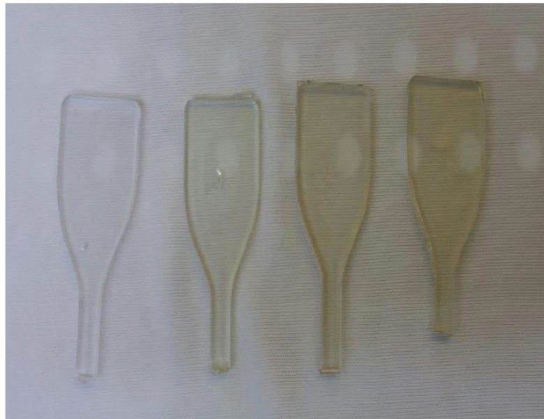
Figure 6: Degraded specimen according to the residence times (from left, 0 min (normal), 60, min, 90 min, 120 min).
