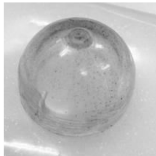
Figure 2: The second case: small inclusions in injection molded specimen.
