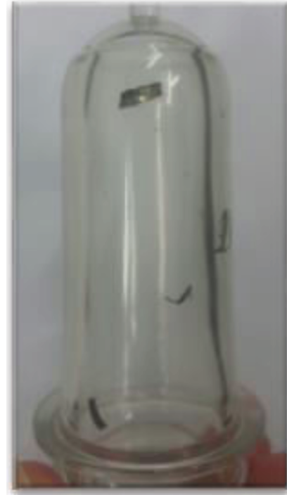
Figure 1: The first case: injection molded blow preform with foreign materials inside.
