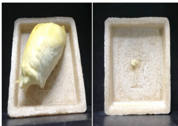
Figure 8: The appearance of packaging produced from composite cassava starch foam trays blended with 10% kraft fiber and 10% gluten protein, a ) before packing minimally processed durian and b ) after packing minimally processed durian.
