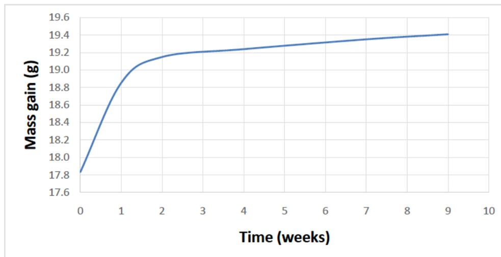
**Figure 3:** Example of the experimental absorption curves showing the evolution of the mass gain as a function of immersion time.
