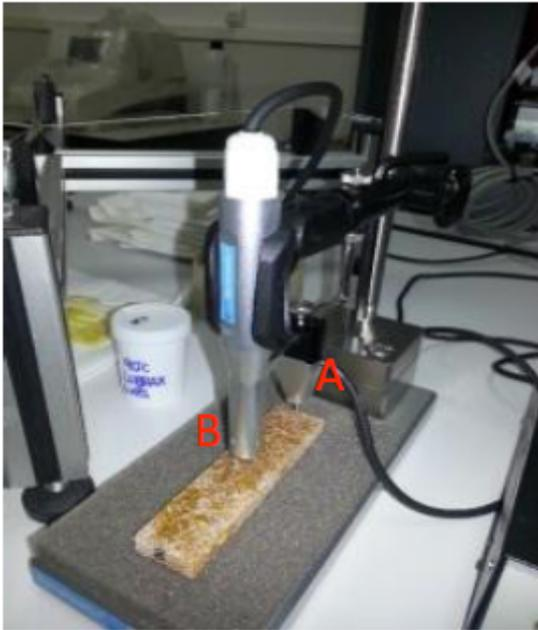
**Figure 2:** Experimental setup for the acoustic test, showing the relative position of the dart (A) and the microphone, (B) in respect to the sample.
