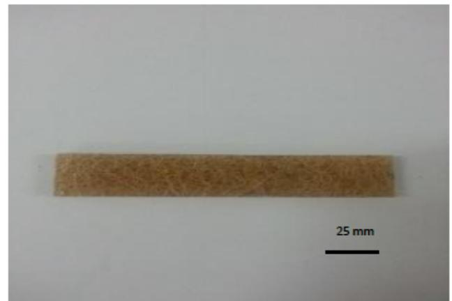
**Figure 1:** Test specimen used for the mechanical, absorption and acoustic characterization.
