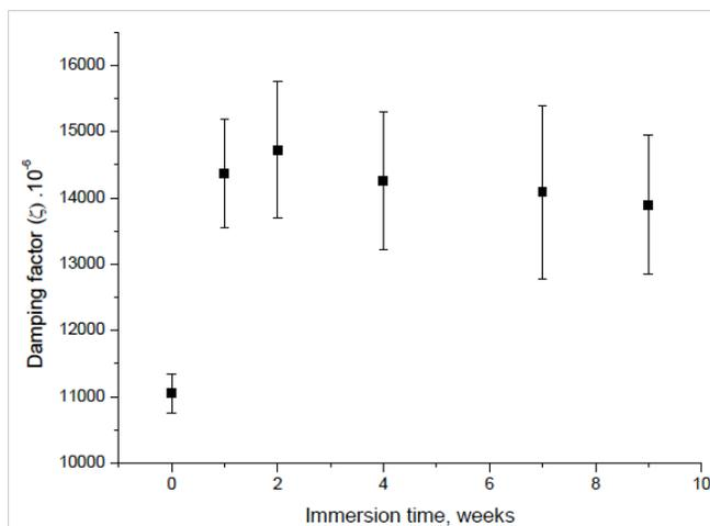
**Figure 6:** Variation of the damping factor ( $\zeta$ ) as a function of immersion time.
