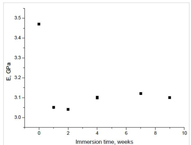
Figure 5: Evolution of the elastic modulus with the time of water absorption. Error bars were placed on the chart but are often too small to be visualized.
