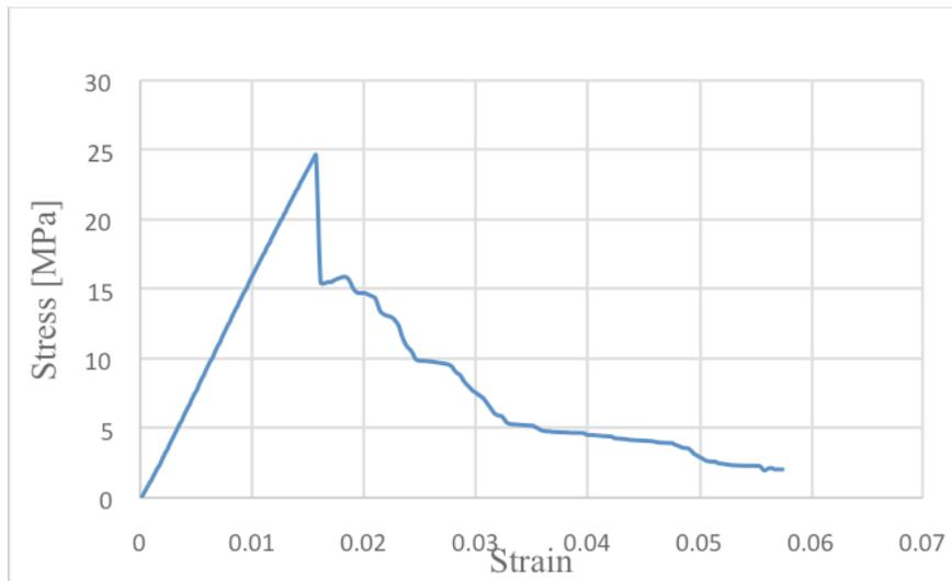
Figure 4: Typical stress-strain curve presented by the composites.
