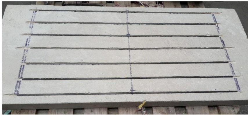
(b) Insertion of CFRP rods into the grooves.
