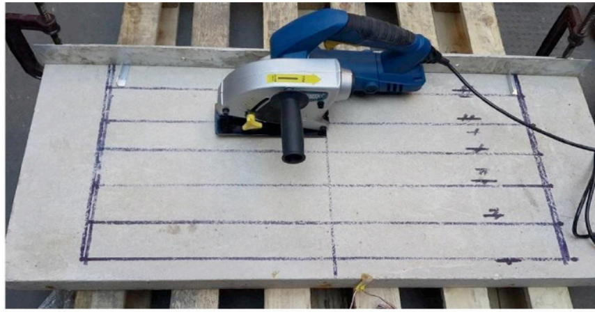
(a) Preparation of grooves using a wall chaser machine.
