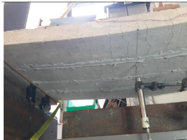
b) Evenly distributed tensile cracks at bottom face of slab QS1
