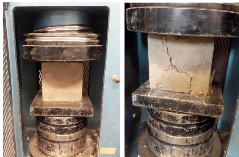
Figure 2: Concrete compressive test of the cubes.
