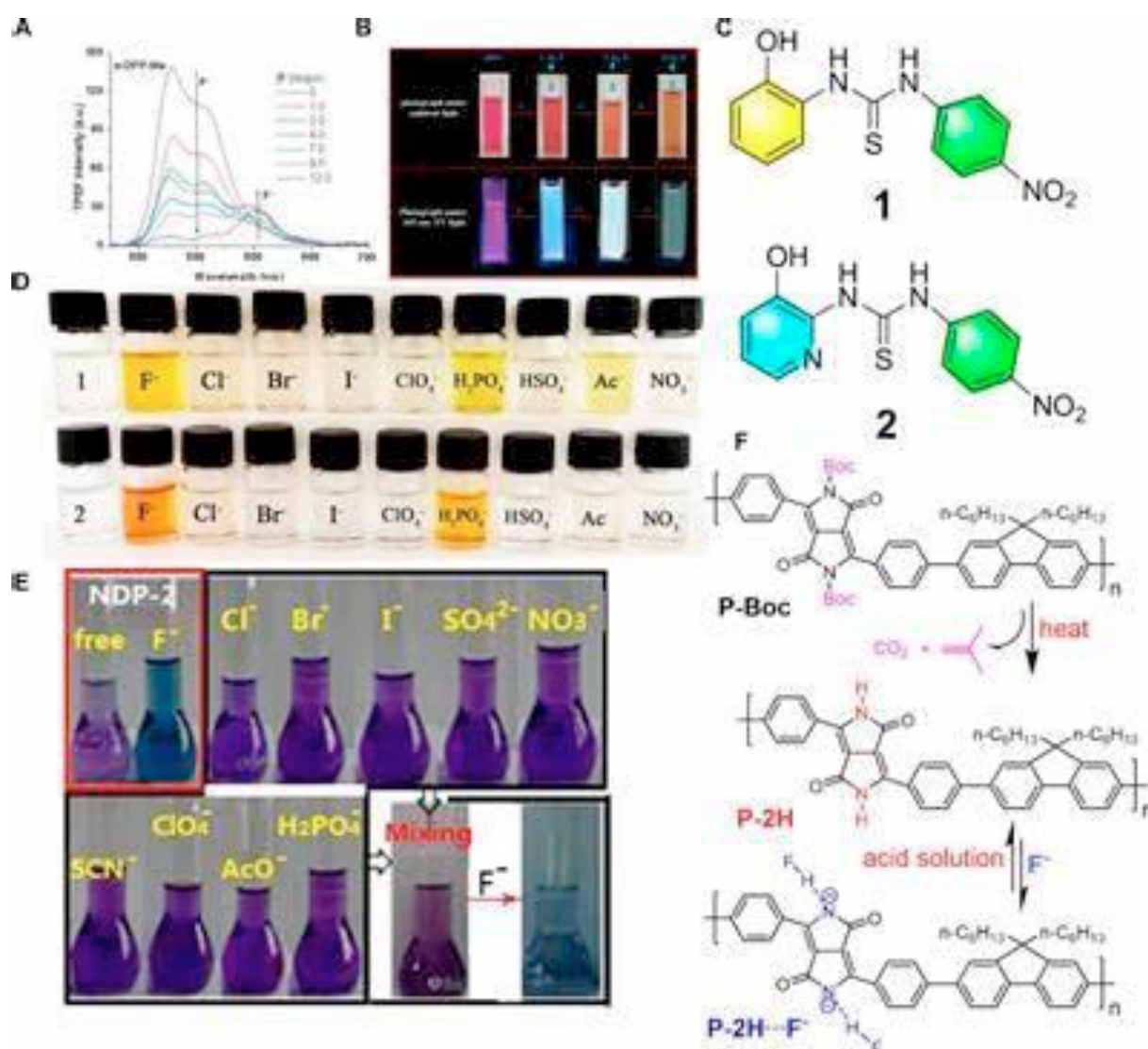
Figure 2: An ion sensor that uses fluorescence to detect fluoride ions [3].
