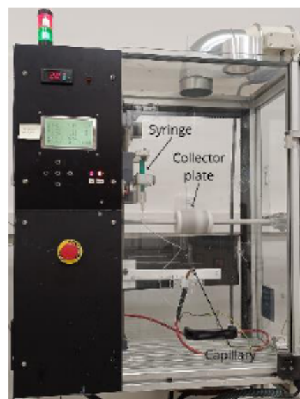
Figure 1: Electrospinning machine from INTEXTER-UPC.
