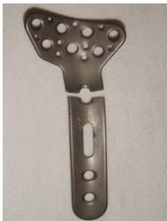
**Figure 7:** Retrieved broken VariAx plate (case 2) demonstrating transverse fracture of the plate at the sides of the screw hole.
