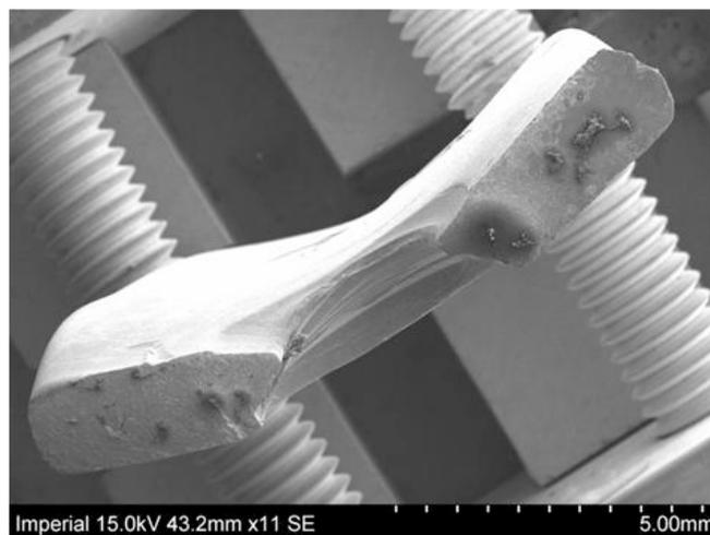
**Figure 8:** Scanning electron microscopy studies showing patterns suggestive of fatigue failure: End-view of fractured plate, with half of the screw hole in cross-section.
