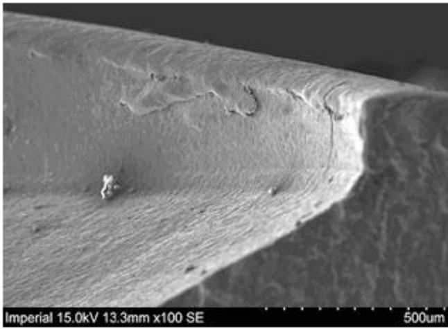
**Figure 10:** Scanning electron microscopy demonstrating damaged edge of screw hole at the top, with deformed metal and a crack near the fracture surface, which is the dark area at bottom, right. The area at the centre, left of the picture is the countersink, where the screw head sits when inserted fully.
