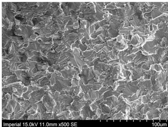
**Figure 9:** Scanning electron microscopy of the fracture surface, showing brittle granular fracture morphology, with numerous grains having fine striated patterns typical of a fatigue process.
